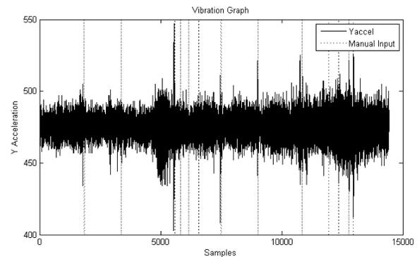
Figure 4: Raw vertical acceleration readings and the manually marked potholes.
