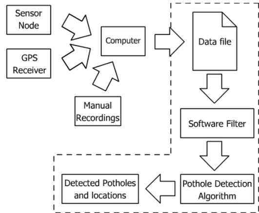
Figure 2: The block diagram of the data collection and the analysis process.
