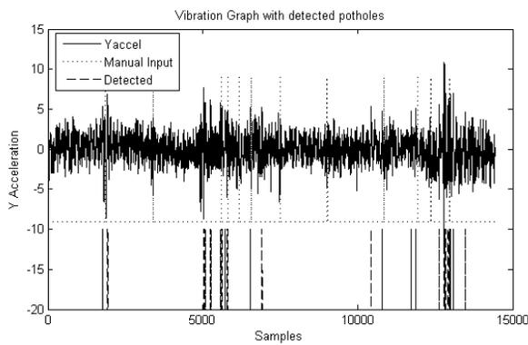
**Figure 6: Auto detected potholes.**
