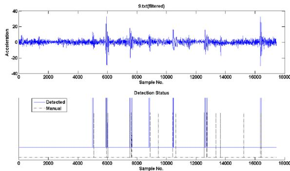
**Figure 7: Auto detected potholes on another stretch of road.**
